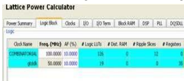
Fig.5. Number of LUTs and registers used by the design on FPGA after place and route.
